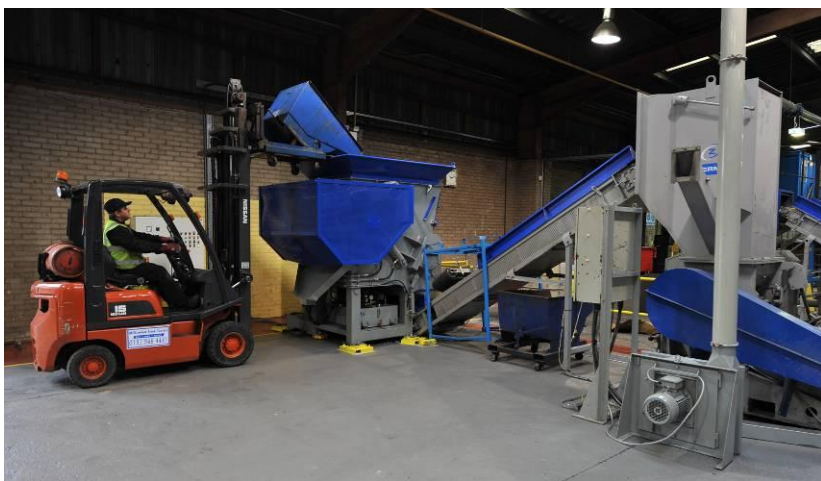
Manual or mechanical loading of the plastic shredders
