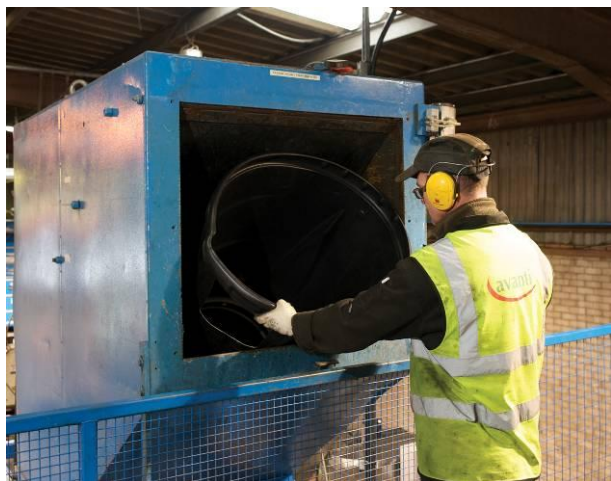
Manual or mechanical loading of the plastic shredders
